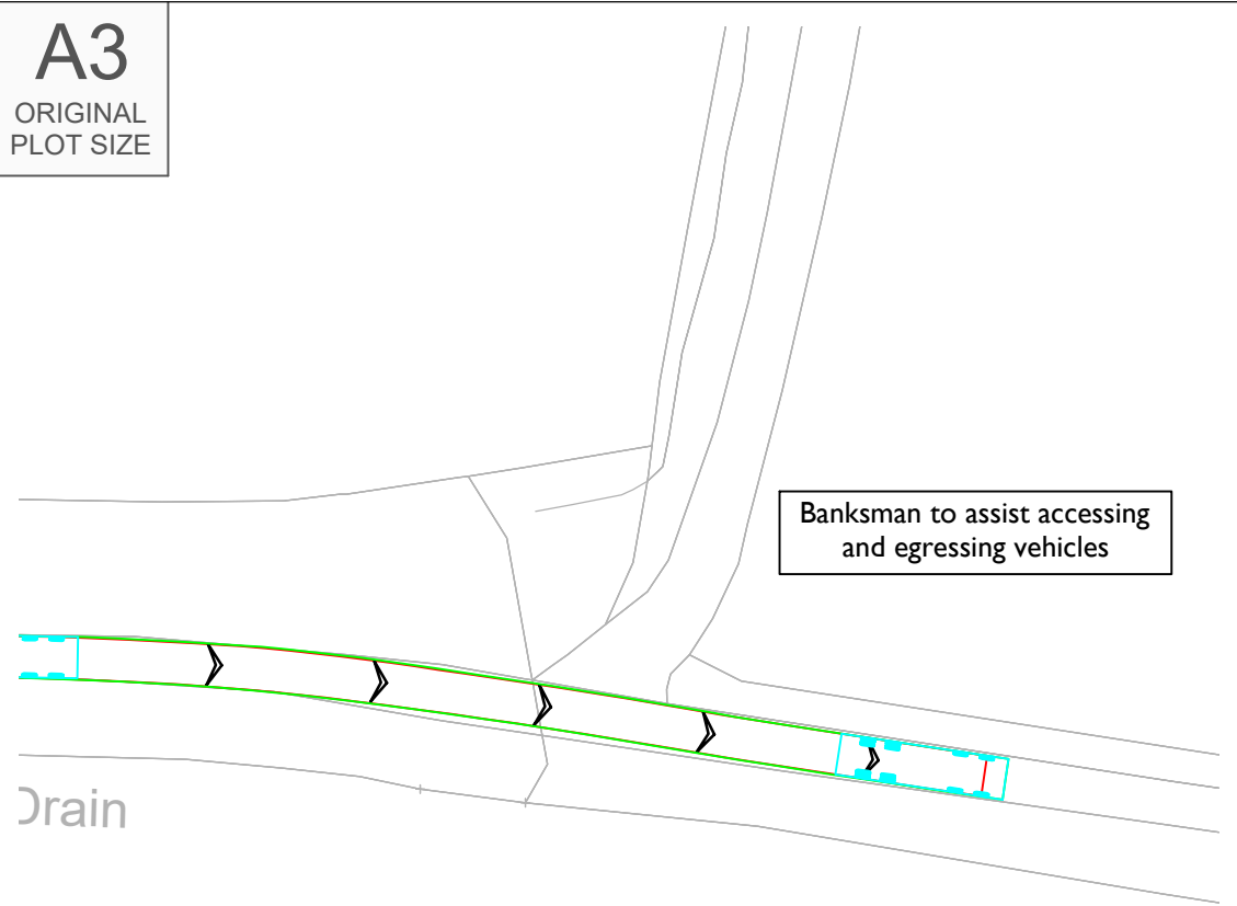
Tipper Vehicle Entering Site
